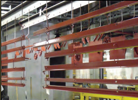
Two-coat system is utilized for proper application of PowderGuard™ Zinc finish
